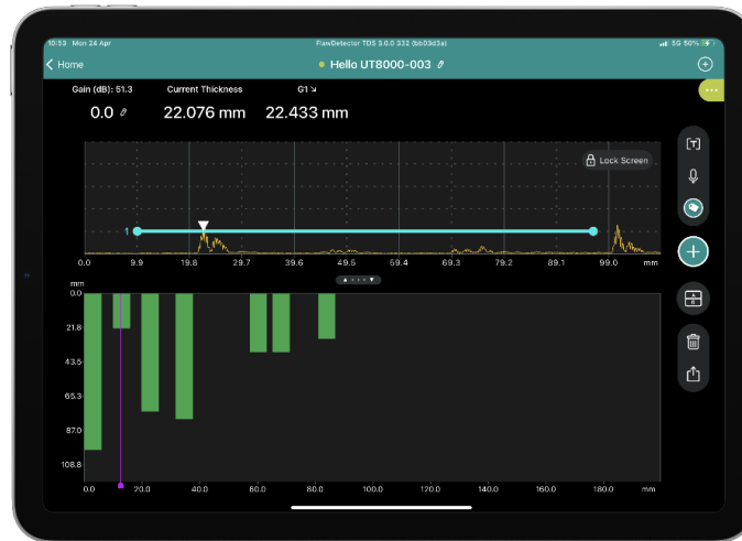
Figure 51: B-Scan post processing, single value
