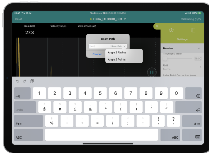
Figure 29 F: Calibration Option with Angle Probe
