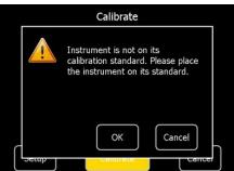
Take care that the ZRM 6013+ is placed correctly on the included calibration standard. Otherwise, the ZRM 6013+ will give you an error message. The instrument has to snap in which is indicated by a click sound.
