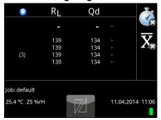
By pressing the measuring button the reading is started. During the measuring period which is about 2-3 seconds, you will see "-" on the top line and the symbol on the top left side.
