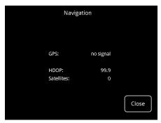
The WAAS GPS-unit is not able to receive a positioning signal. The coordinates cannot be displayed.
