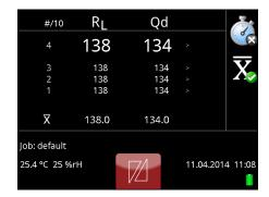
The single values are still displayed. On the left side of the page the measurements are numbered. On the bottom line you see the symbol for the average
