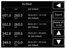
In the first column you see the  $R_L$ -values and in the second column the Qd-values. In the third column there are listed the date, time, the number of single measurements e.g. (5) at average measurements as well as the job. Press on a desired line for getting some additional information to the entry.
