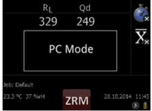
Connect the ZRM 6013+ with a USB-cable to a computer. The message "PC Mode" should appear on the touchscreen of the ZRM 6013+.
