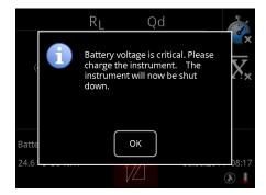
In order to prevent a damage of the battery, the instrument switches automatically off before the battery is completely empty. The ZRM 6013+ announces this by displaying the symbol of an empty
