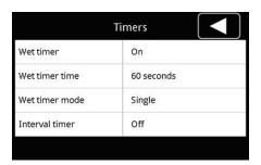
If the wet timer is activated, you can see the current setting for the wet timer time and wet timer mode. For changing these settings, you need to press on the respective line.
