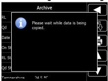
pressing the button all measuring entries will be stored on the USB-stick. The message beside will be shown during copying. The exported measurements can be opened on a computer/laptop using the mapping software "MappingTools". The Use of MappingTools is described in the separate instruction
