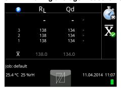
For activating average reading press on the touchscreen the symbol . If the symbol is shown, the average reading is activated.
