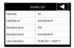
Please check the calibration settings also for the Qd geometry and if necessary change them accordingly.
