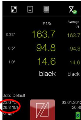
The used illumination angle is always shown in the display of the main view and this information is stored to each measurement.
