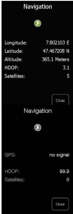
After switching on the ZRS 6060, connecting the WAAS GPS unit can take up to 15 minutes until the unit is receiving coordinates. Ensure clear view to the sky to receive good signals.
