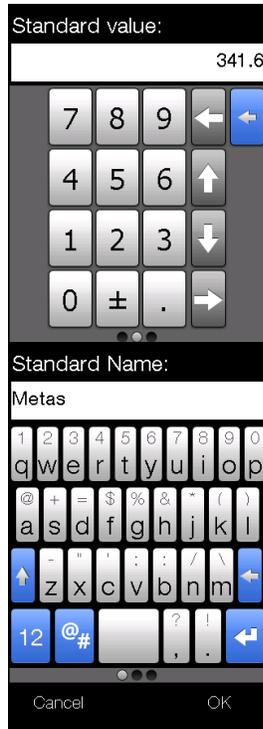
Here the value of the second standard can be inserted. This might be a known reference value of an internal sample or a value measured by an official institute. After the input has been confirmed by tapping „OK“, the menu item „calibration settings“ will be displayed automatically.
