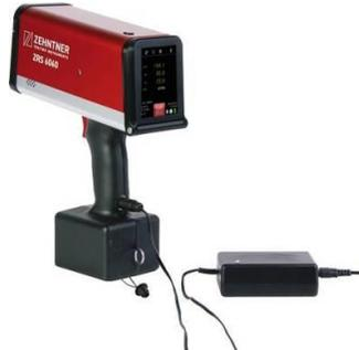
To charge the battery, plug the charger plug into the socket on the ZRS 6060 and connect the charger to a wall socket (100 – 240 V, 50 - 60 Hz). The special plug on the charger has a reverse polarity protection. The unit can be used and turned off or on while charging. For disconnecting the charger press on the “push button” on the plug of the battery charger.
