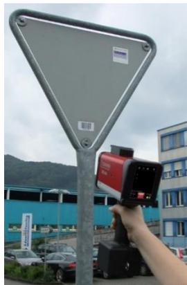
Before triggering a measurement the barcode needs to be read. Switch on the ZRS 6060 and place it closely to the barcode and lift it up and down until the barcode is recognised by the barcode reader.
