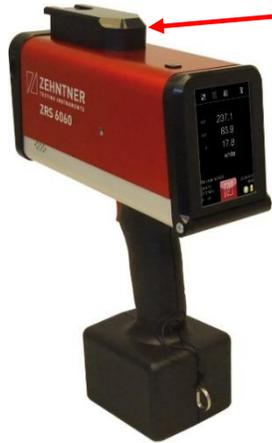
The ZRS 6060 can be equipped with a barcode reader or with a QR barcode reader. Both will be mounted on the top of the ZRS 6060.
