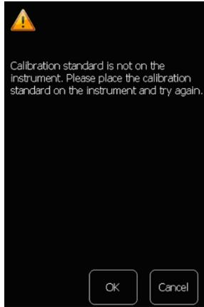
Make sure that the front plate with the calibration standard is placed correctly. It needs to be mounted in the calibration position, otherwise an error message will be displayed. The front plate has to latch audibly.
