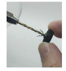
Put a small amount of CA Glue around the outside of the 2.3mm bushing tube, spin and push the bushing into the wheel until it bottoms out. Allow to dry for at least 10 minutes. After 10 minutes, the bushing should be locked in place and will not turn.
