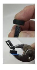
wheel still spins freely. Again making sure that the spindle is going in straight and the wheel spins true. Repeat for the other side.
