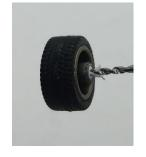
Once the rear wheels have the correct hole size, test fit and trim the shaft to attain the right overall width, which will be the same as the front "overall width". When installing or removing the wheels from the axle always use the needle nose pliers. If you force the axle to turn it will damage the gears.
