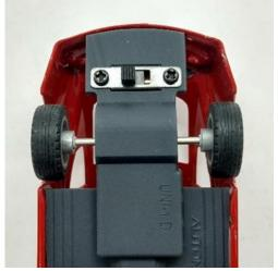
**Front axle spindle sizing**. The front axle spindle size is 1mm. The hole size in the wheel needs to be the same size. Wheel hole sizes vary widely but are rarely larger than 2.2mm.
