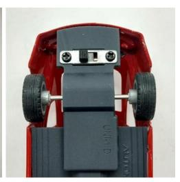
**Front axle spindle sizing**. The front axle spindle size is 1mm. The hole size in the wheel needs to be the same size. Wheel hole sizes vary widely but are rarely larger than 1.5mm.
