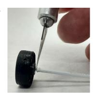
B. Tighten the 1mm drill bit into the pin vise and carefully spin the wheel around the drill bit. Be sure to spin it true and stop when it bottoms out. Be careful not to go all the way through the wheel. Your wheel is now the correct size and ready to install onto the spindle.
