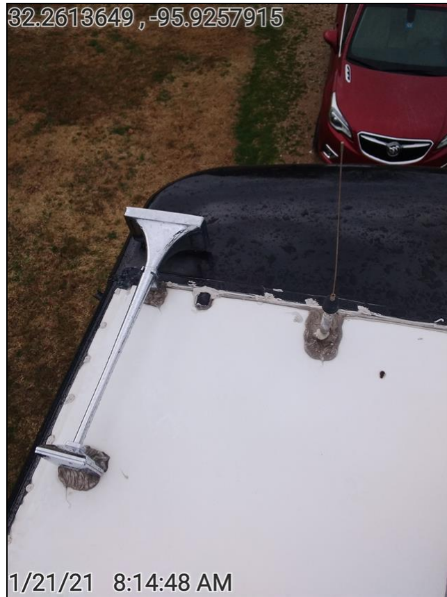
Streetside air horn, CB Antenna and satellite radio antenna
