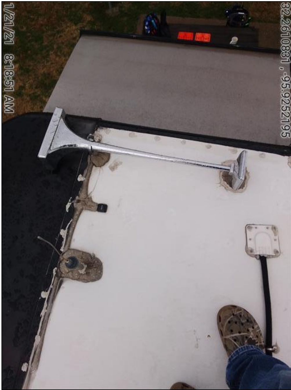
Curbside air horn, GPS antenna and cockpit radio antenna
