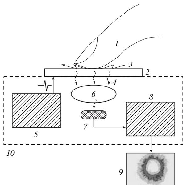
**Fig. 2.** Scheme of the GDV device. (1) Object of examination; (2) transparent electrode; (3) gas discharge; (4) optical emission; (5) generator; (6) optical system; (7, 8) video transformer; (9) computer; (10) case.
