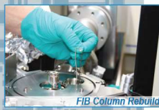
FIB Column Rebuild
