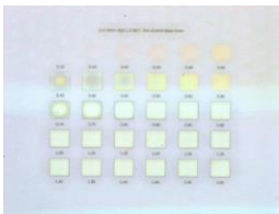
WITH DisCharge: no charge accumulation. Structure appears as expected with no harm to PDMS.
