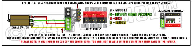
WITH EITHER INSTALLATION OPTION YOU CAN REVERSE THE RED OR YELLOW WIRE TO CHANGE THE SELECTOR SWITCH ORIENTATION WITHOUT THE NEED TO REMOVE IT FROM THE GUITAR.
