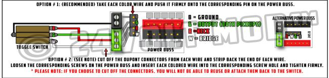
WITH EITHER INSTALLATION OPTION YOU CAN REVERSE THE RED OR YELLOW WIRE TO CHANGE THE SELECTOR SWITCH ORIENTATION WITHOUT THE NEED TO REMOVE IT FROM THE GUITAR.
