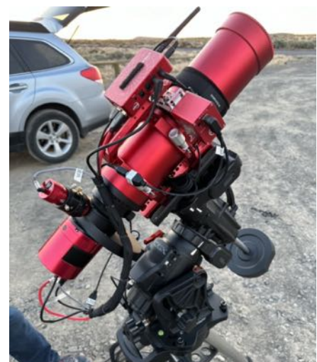
Chris Hill's Wide Field Photographic Telescope 2.75" Petzval Refractor with 26MP Cooled Colored Camera
