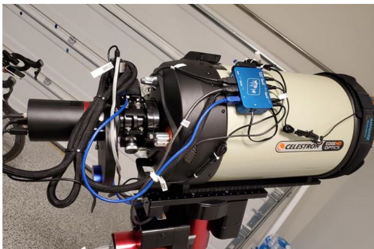
Chris Hill's Long Focal Length Photographic Telescope 11" Corrected Schmidt Cassegrain with a 60MP Cooled Mono Camera
