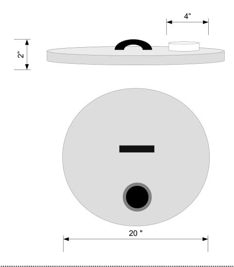
Our durable concrete lids are designed to securely cover our current style of concrete tanks. Fitted with a heavy duty plastic handle that does not rust or corrode. Each lid features a built-in 4" coupling, allowing customers to easily extend a pipe to the surface for self-monitoring or other needs. Built to last and easy to install, these lids offer a practical solution for a wide range of applications. For additional options or customizations, give us a call.
