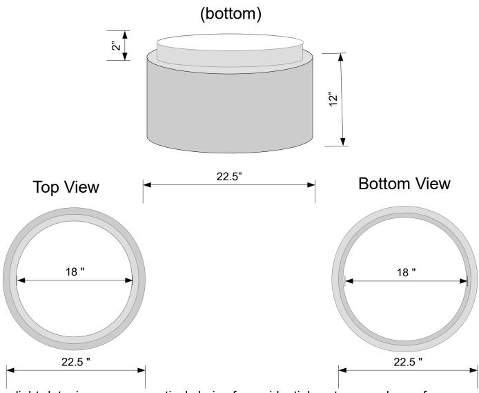
Our light-duty risers are a practical choice for residential customers who prefer an alternative to plastic risers. Designed to extend concrete tank openings to the surface, they can be fitted with a durable concrete lid for a clean, secure finish. While perfect for many applications, please note that these risers may not meet code requirements for new installations in certain counties. For questions or custom solutions, please call.
