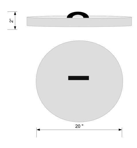
Our durable concrete lids are designed to securely cover both standard and bottomless distribution boxes. Each lid is fitted with a heavy-duty plastic handle, ensuring long-lasting performance without the risk of rust. Built for ease of use and reliability, these covers provide the perfect finishing touch for your distribution box installation.
