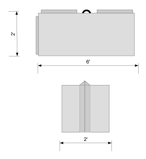
Our heavy-duty concrete retaining wall blocks offer a quick and reliable solution for retaining walls. Measuring 6 feet long, 2 feet tall, and 2 feet thick, each interlocking block weighs approx 3,000 lbs, ensuring stability and durability. Designed to stack up to three high, these blocks are perfect for creating sturdy walls in a fraction of the time. For more information or to discuss your project needs, give us a call.
