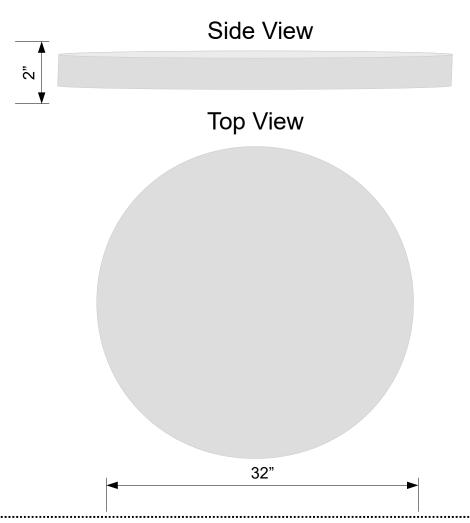
Our heavy-duty concrete cover is designed to cover our heavy-duty concrete risers. This is a less expensive alternative to a cast iron manhole cover. These are not advised for constant traffic on them but are heavy duty enough for occasional use.
