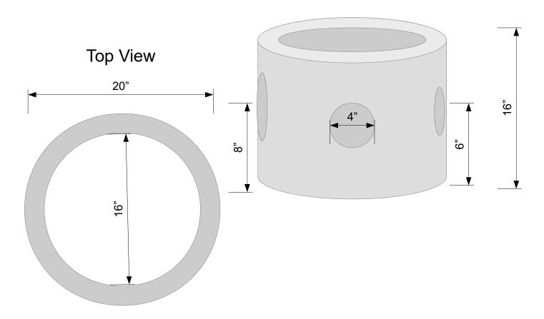
Our bottomless distribution boxes are an ideal solution for dry well leach line installations, providing effective and reliable gravity flow management. Designed with the same versatility as our standard distribution boxes, this model features a bottomless design for enhanced drainage. With up to four knockouts for easy on-site configuration, these boxes are built for durability and adaptability. For questions or custom options, give us a call.
