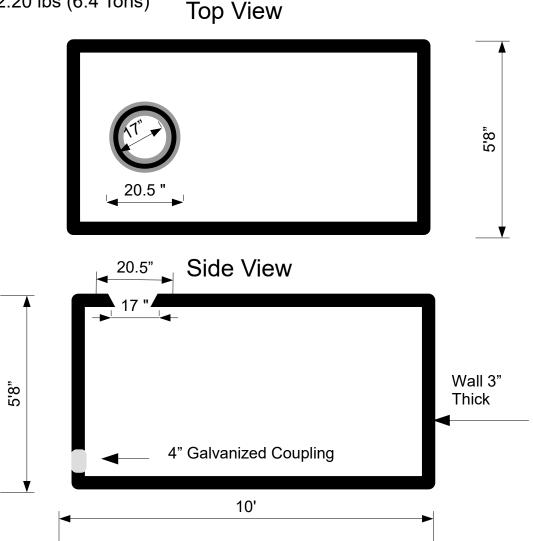
Our high-quality concrete water tanks for reliable water storage, ideal for fire suppression, rainwater harvesting, irrigation systems, well solutions, and more. Built to last, designed to perform. Comes with one lid opening with cover and a 4" galvanized coupling so that multiple tanks can be tied together.
