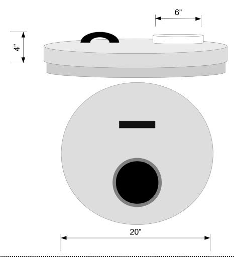
Our durable concrete lids are designed to securely cover our concrete tanks while providing added functionality. Each lid features a built-in 6" PVC pipe, allowing customers to easily extend a pipe to the surface for self-monitoring or other needs. Built to last and easy to install, these lids offer a practical solution for a wide range of applications. For additional options or customizations, give us a call.
