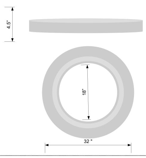
Our versatile concrete rings are the perfect solution for repairing or converting tank openings that are degraded or uniquely sized. Designed to install on top of the tank, these rings create a secure, standardized opening that accommodates our normal concrete lids. Durable and easy to install, they ensure a long-lasting fit and functionality for your tank. For more information or assistance, give us a call.
