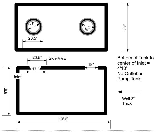
Our durable concrete pump tanks are designed as single-compartment holding tanks for pumping water or wastewater. Featuring a single inlet opening and two top openings fitted with our concrete lids and PRTA compatibility, these tanks are ready to accept Orenco risers. Built for reliability and ease of use, our pump tanks provide a practical solution for residential and commercial pumping systems. For more details or assistance, give us a call.
