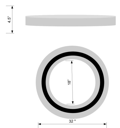
Our concrete rings with PRTA provide a practical solution for repairing or converting tank openings that are degraded or uniquely sized. This design allows for easy installation of a common Orenco riser on top of the ring, offering seamless compatibility and versatility. Durable and functional, these rings ensure a secure fit and long-lasting performance. For more details or assistance, give us a call.
