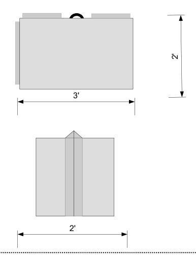
Our 3-foot concrete retaining wall blocks are the perfect complement to our larger 6-foot blocks, allowing you to offset seams and enhance the structural integrity of your retaining wall. With the same durable design and 2-foot height and thickness, these 1,500-lb blocks provide stability and versatility for your project. For more details or assistance with your retaining wall plans, give us a call.
