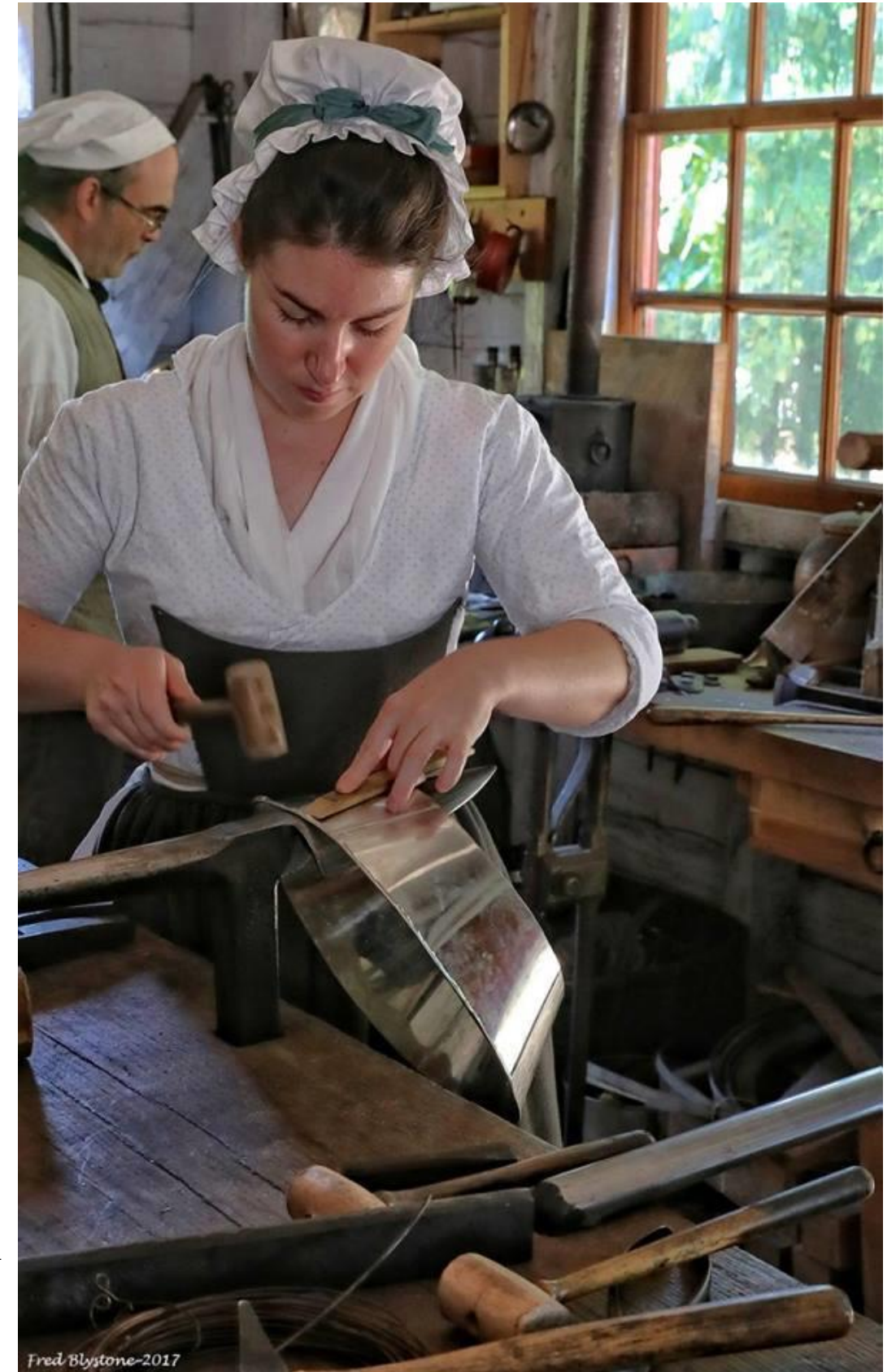
Right: Working on a milk pan for Historic Foodways. Steve Delisle, journeyman tinsmith (and my supervisor), in the background.
