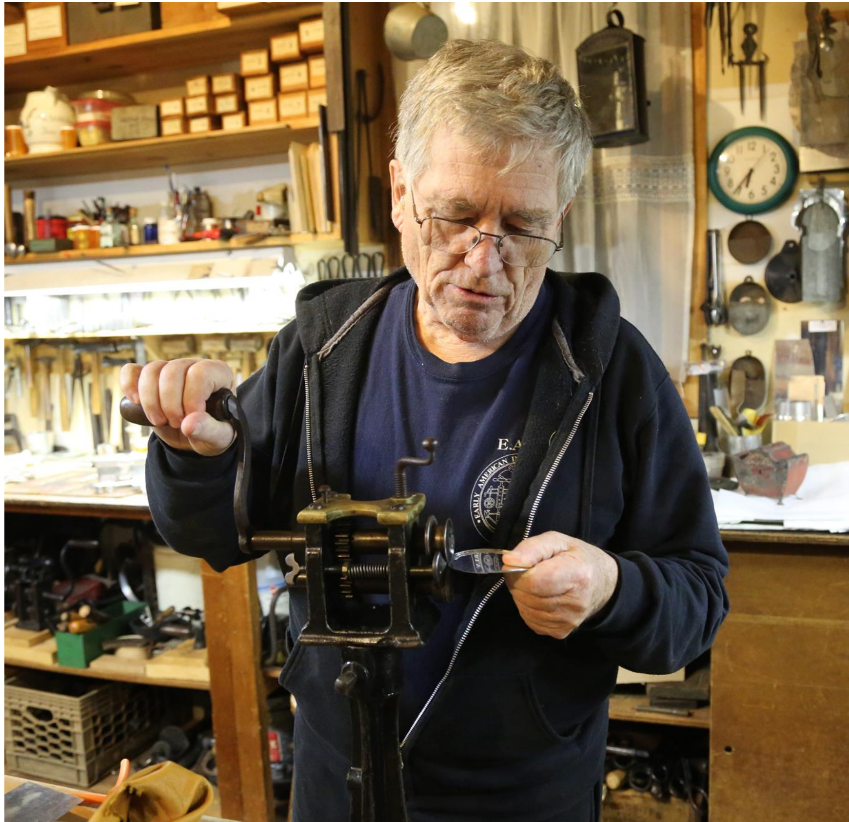
Right: Fleur-de-lis sconces, Bill's first tinsmithing project at Historic Eastfield Village in 1976. Above: Bill demonstrating one of the first tinner's machines he purchased, a burring machine.
