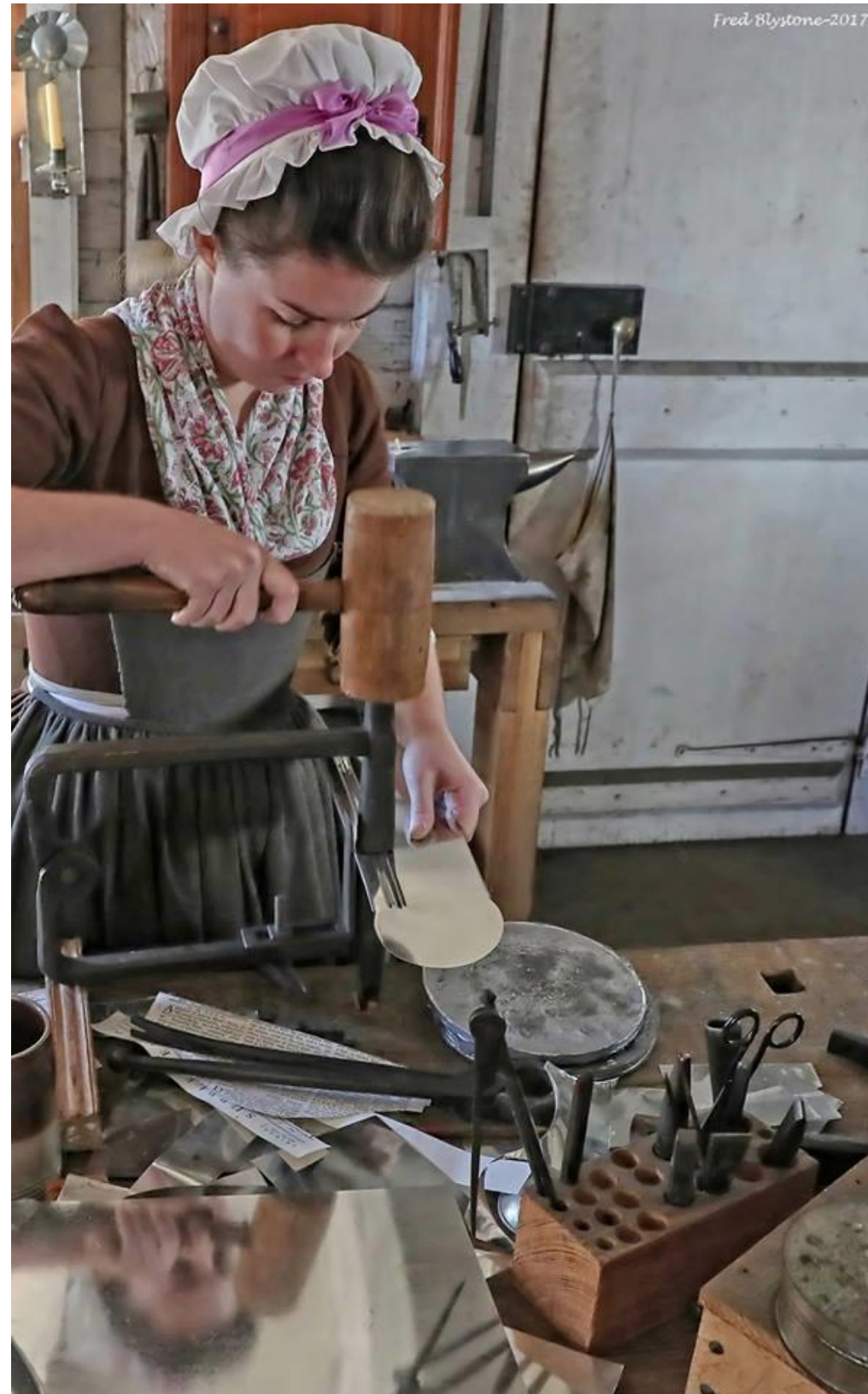
Using a cullender swedge to shape a wall sconce.
