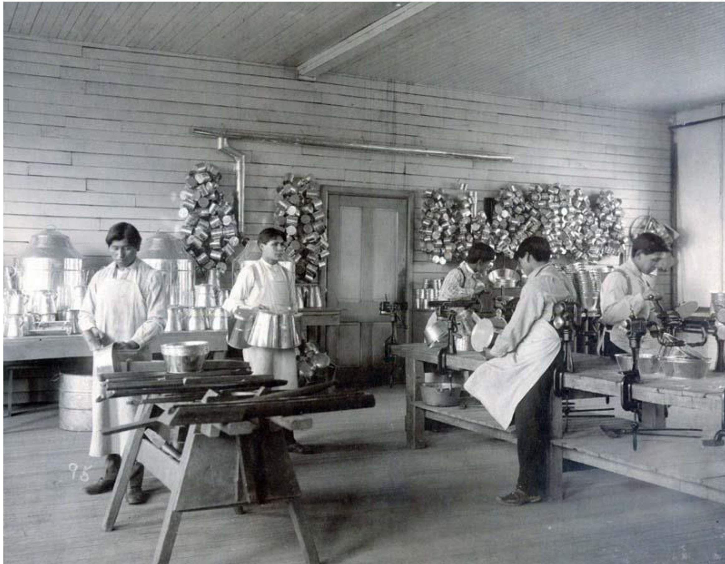
View of the tin shop with students at work in 1901 showing tinner's stakes and machines used by the students. Note the wall of cups in the background.
