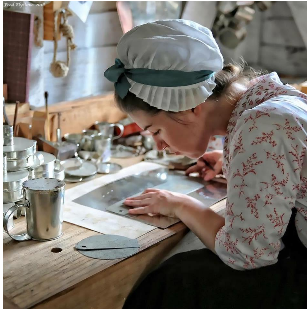
At my Colonial Williamsburg tin shop work bench, tracing out a cup pattern onto tinplate. All photos in this article courtesy of Fred Blystone.
