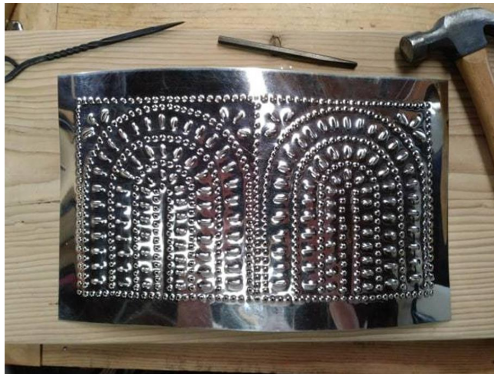
Figure . The recreated back of the lantern. The panel of tinplate is 8.5 inches by 14 inches overall.
