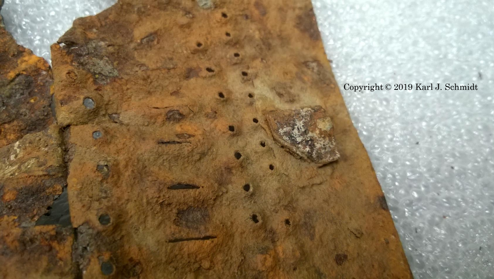
Close-up of lantern body, showing the catch, which has been crushed.
