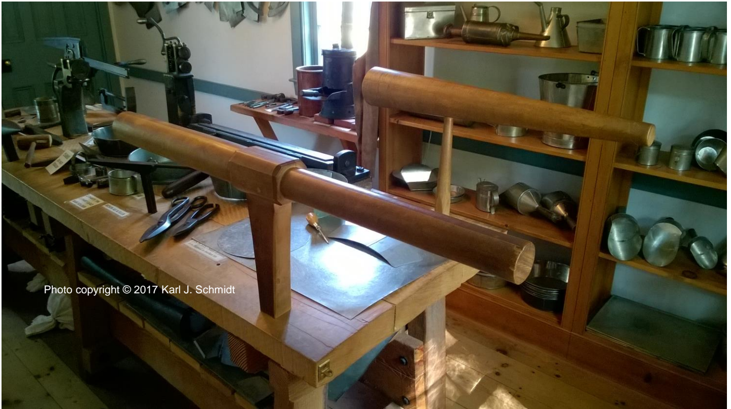
ABOVE: View of the workbench, showing the wooden conductor stake and wooden mandrel, used for shaping tinplate.
