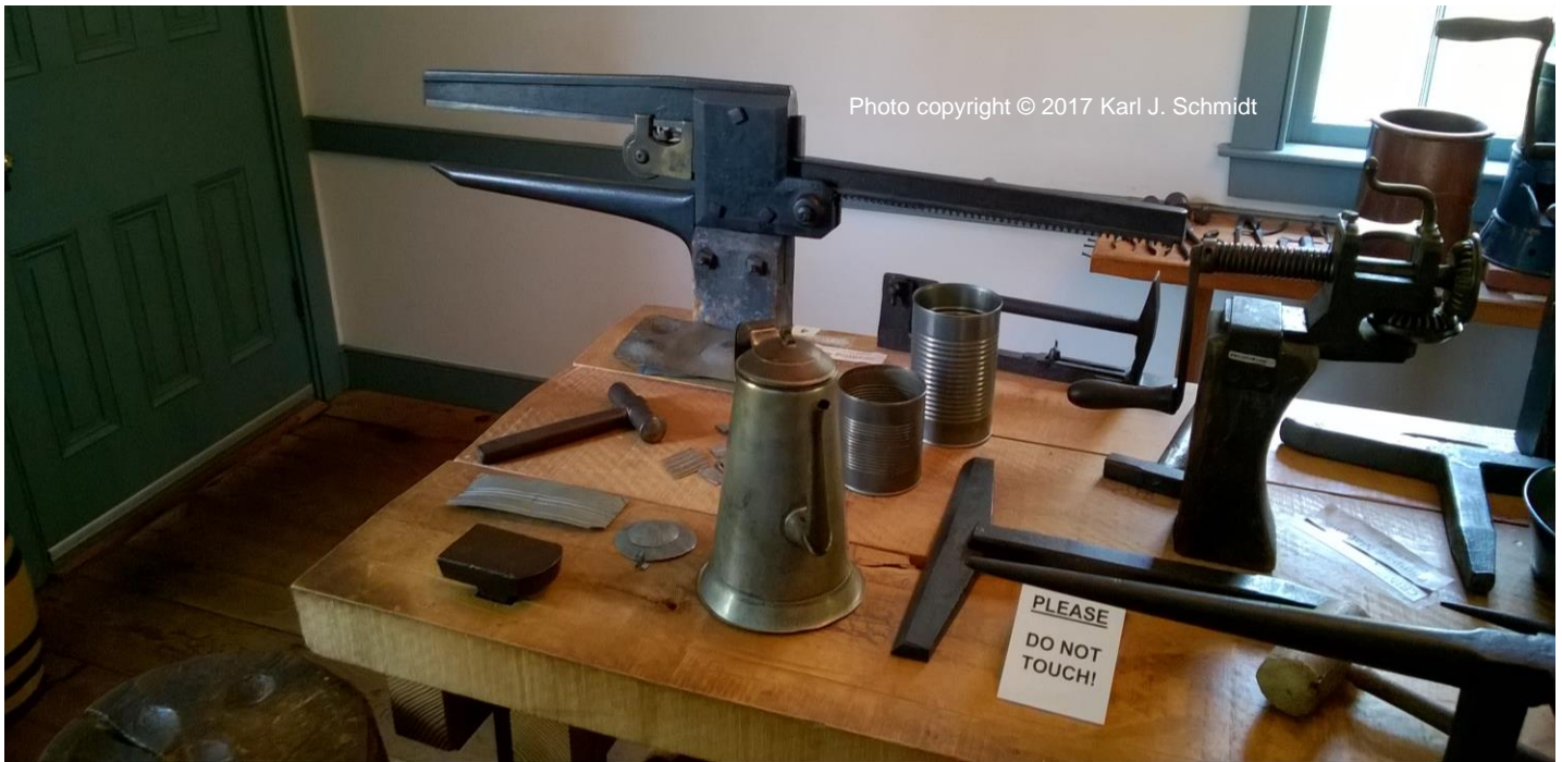
ABOVE: Stoddard tin shop workbench, showing some of the tools and machines on display, including a setting down machine (right) and a grooving machine (left). A hatchet stake and a creasing stake can be seen lying down on the workbench, while a square pan swedge can be seen on the far side of the workbench. A raising hammer can be seen at the end of the bench. BELOW: Some of the patterns on display in the Stoddard tin shop, hanging on nails against one wall. They include patterns for flared pans, bread bowls, and coffee pots.
