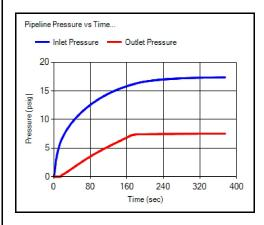
**Graphic Results** - GASPurge displays its results in a graphic chart to visualize the pipeline purging process conveniently. Users can view Flow Rate versus Time, Pressure versus Time, Pipeline Velocity versus Time, and Exit Velocity versus Time.
