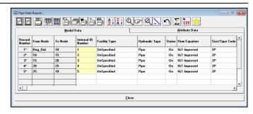
pressures, flow rates, velocities and volumes, and simultaneous reporting of linear and pressure drop per User specified length. Selection sets may be created from within the data reports, allowing unique reporting of User specified data groups. Hierarchical gueries allow the creation of sub-sets from a previously created selection set.
