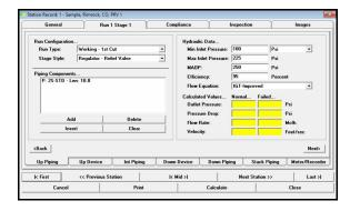
An "audit" screen is provided to allow view-only access to select data. This feature is intended to allow a non-User to view station compliance values while denying the ability to change the data.
