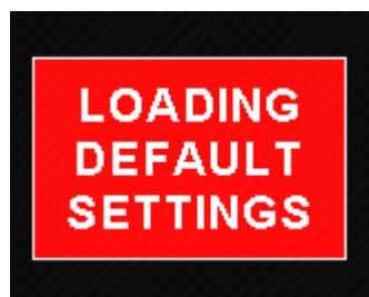
Press and hold the F1/Up button and rotary control during power up to load the pre-programmed factory default settings. The following screen will be displayed:
