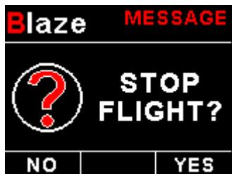
Press the F1/Up button during the normal display mode to manually start/stop a flight. This key is only active if the ASI-5 is setup to select the manual flight option under the "TIMERS" setup menu.
