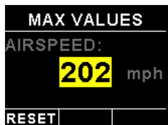
This display can be accessed by rotating the rotary control during the normal display mode. Press the F1/Up button when the max values display is showing to reset the maximum values to the current airspeed.
