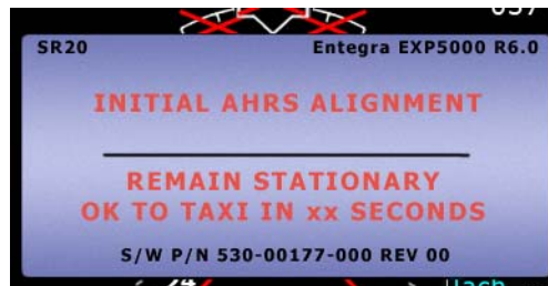
Figure 7. Entegra EXP5000 AHRS Alignment Message
