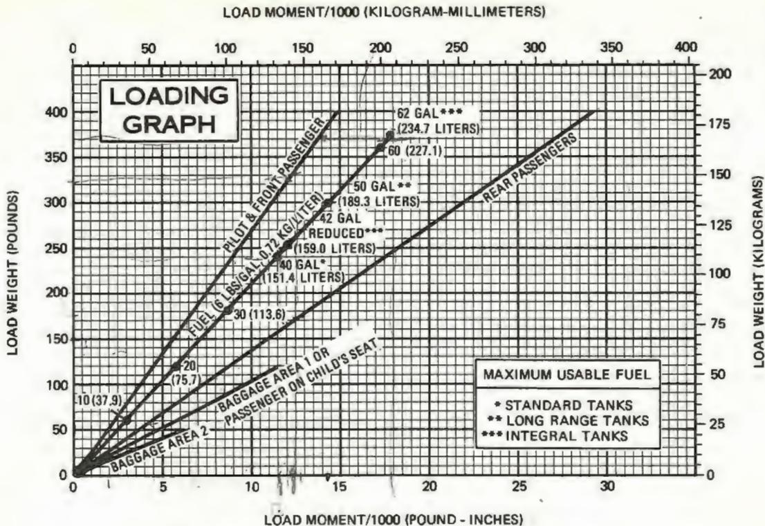
NOTE: Line representing adjustable seats shows the pilot or passenger center of gravity on adjustable seats positioned for an average occupant. Refer to the Loading Arrangements diagram for forward and aft limits of occupant C.G. range.
