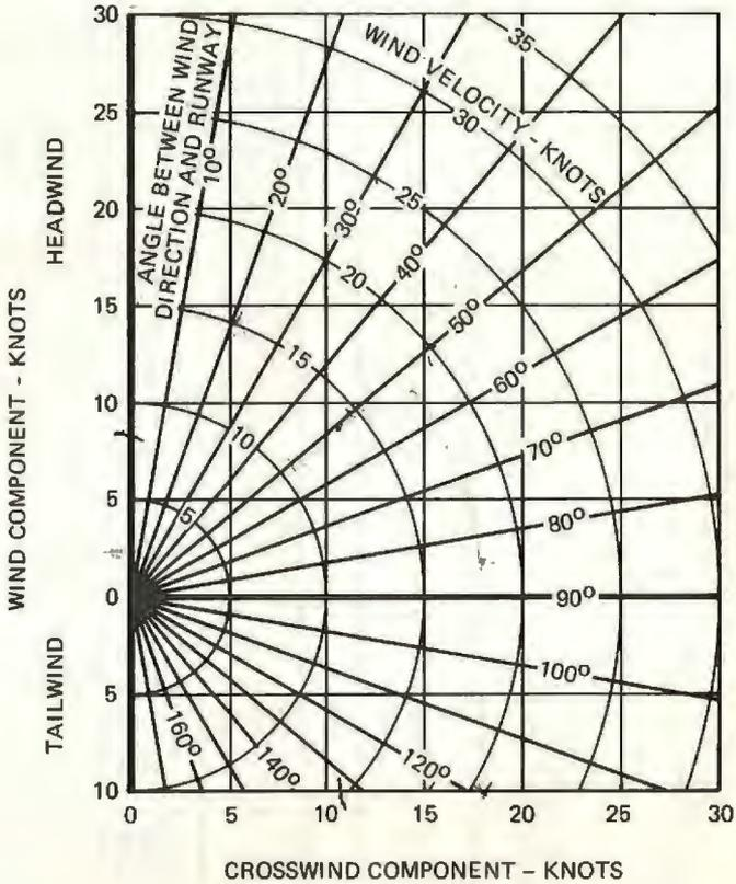
Figure 5-4. Wind Components
