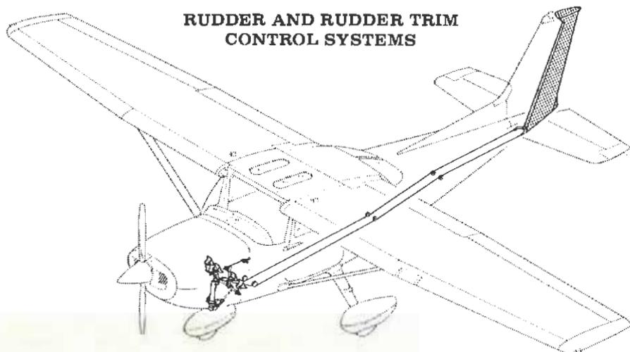
Figure 7-1. Flight Control and Trim Systems (Sheet 1 of 2)
