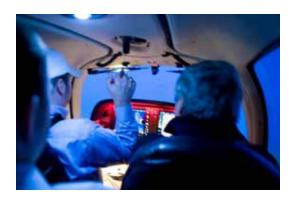
**CAPS Activation** - To activate the CAPS system, the pilot or occupant removes the CAPS activation handle cover and pulls the red handle located in the ceiling between the pilot and co-pilot. The handle should be pulled with both hands in a steady, deliberate, chin up motion. About 45 lbs (20.45 kilograms) of force and two inches of travel are required to activate the system.
