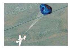
Parachute Disreef – At the beginning of the deployment sequence, the slider ring is positioned at the top of the suspension lines, near the canopy. As inflation loads increase, the slider moves down the suspension lines, allowing the canopy to fully inflate. During the inflation process, the airplane will transition from a nose-high attitude to a nose-low attitude, until the line cutters extend the aft harness to its full length.
