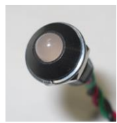
Remote Annunciator Light (RAL)
