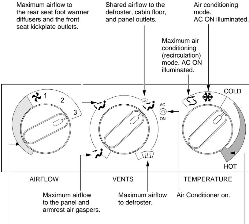
Rotating the selector controls the volume of airflow allowed into the cabin distribution system by opening and closing a butterfly valve in the distribution manifold. When the selector dial exceeds the full open position, the 3-speed blower fan is turned on.
