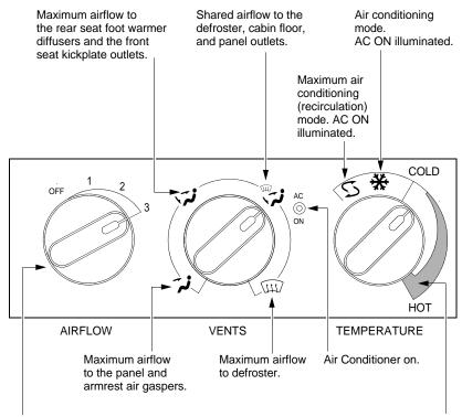
Rotating the selector controls the volume of airflow allowed into the cabin distribution system through use of an electro-mechanical linkage to a butterfly (hot air) valve in the mixing chamber on the forward firewall. When the airflow selector fan speed is moved to the 1, 2, or 3 position the electro-mechanical linkage actuates the hot air valve to the full open position and the 3-speed blower fan is turned on.
