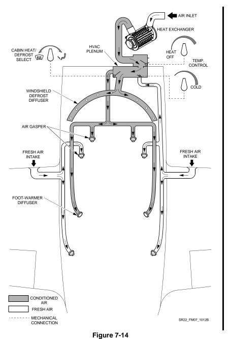
Cabin Heating and Cooling - Serials 0002 thru 1862\*
