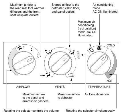
system by opening and closing a butterfly valve in the distribution manifold. (r. When the selector dial exceeds the full open position, the 3-speed blower fan is turned on.
