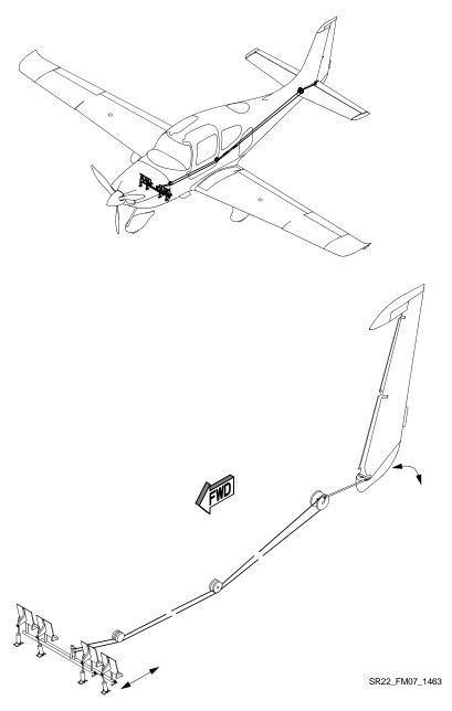
Figure 7-3 Rudder Control System
