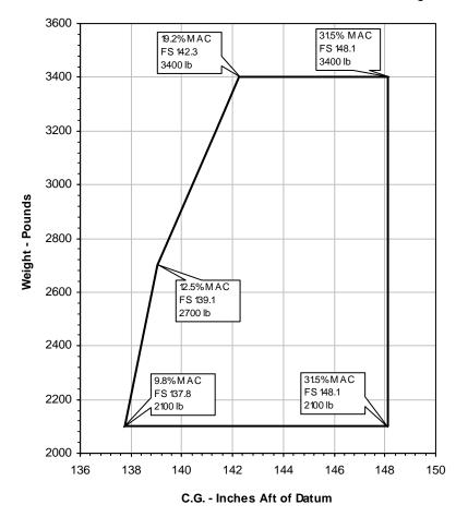
FORWARD LIMIT - The forward limit is FS 137.8 (9.8% MAC) at 2100 lb, with straight line taper to FS 139.1 (12.5% MAC) at 2700 lb, to FS 142.3 (19.2% MAC at 3400 lb.
