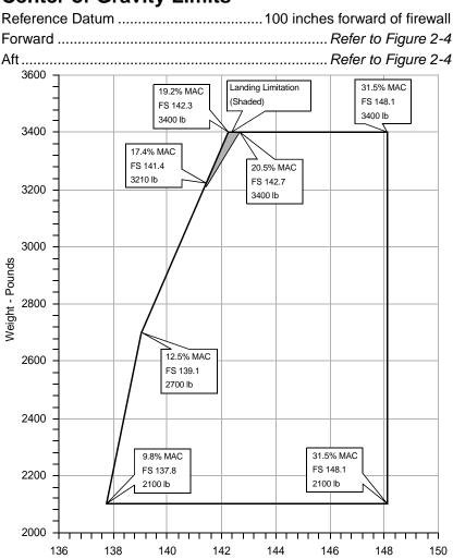
FORWARD LIMIT - The forward limit is FS 137.8 (9.8% MAC) at 2100 lb, with straight line taper to FS 139.1 (12.5% MAC) at 2700 lb, to FS 142.3 (19.2% MAC) at 3400 lb.
