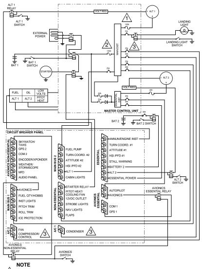
Serials 0002 thru 1601, 1603 thru 1643 and 1645 thru 1662: 80A fuse.
