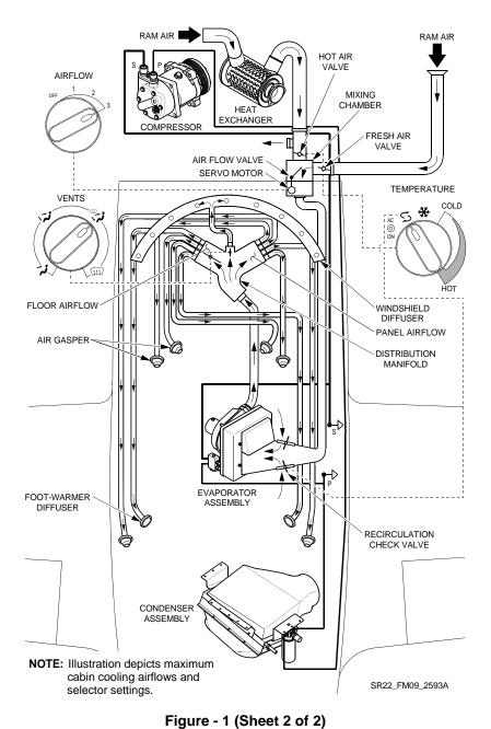
Air Conditioning System Schematic - Serials G3 and Subs
