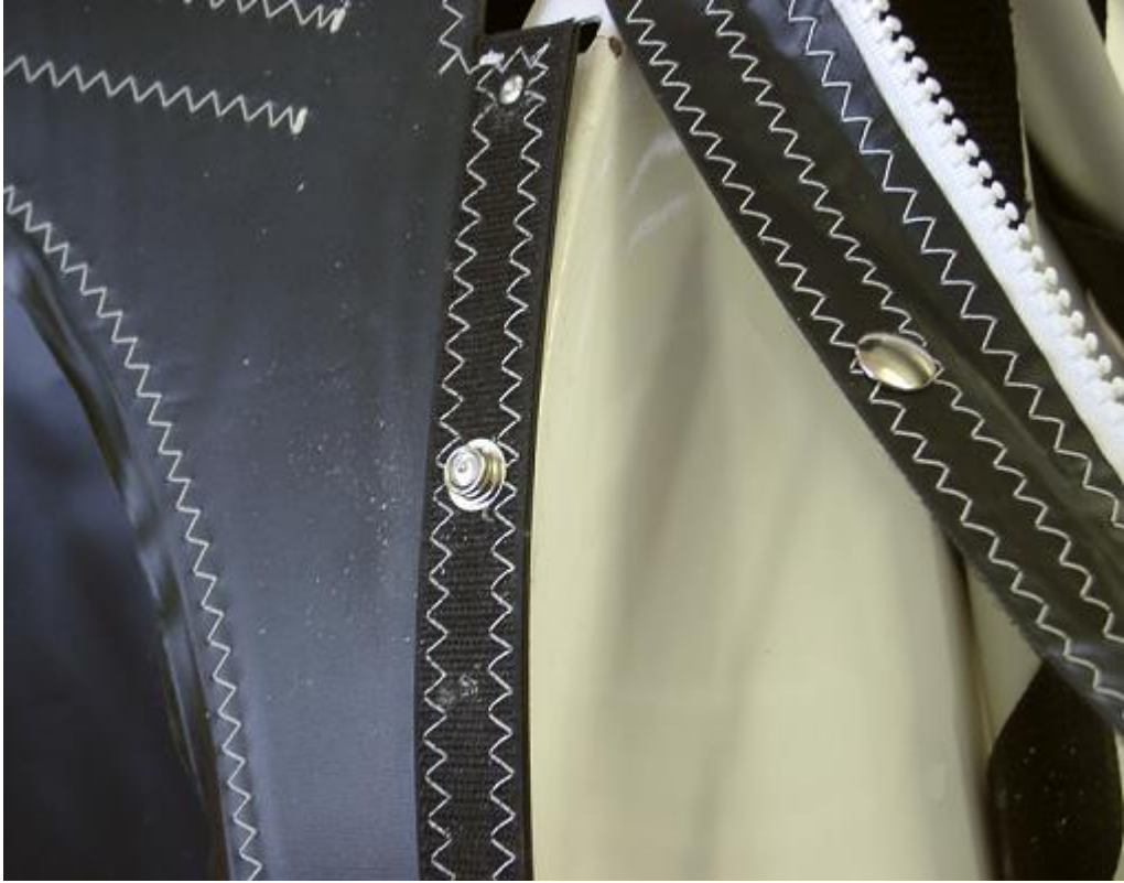
Figure 16 – Snaps Mounted to Bulkhead
