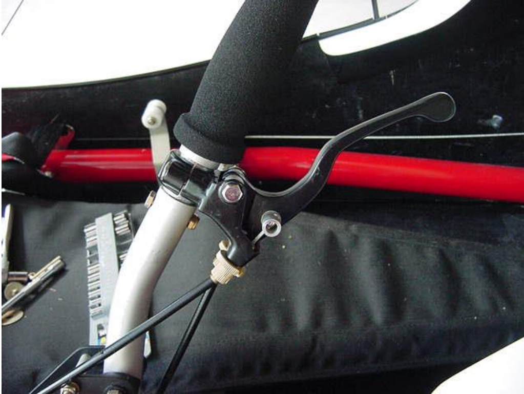
Figure 6 – Assemble Control Stick with Brake Lever
