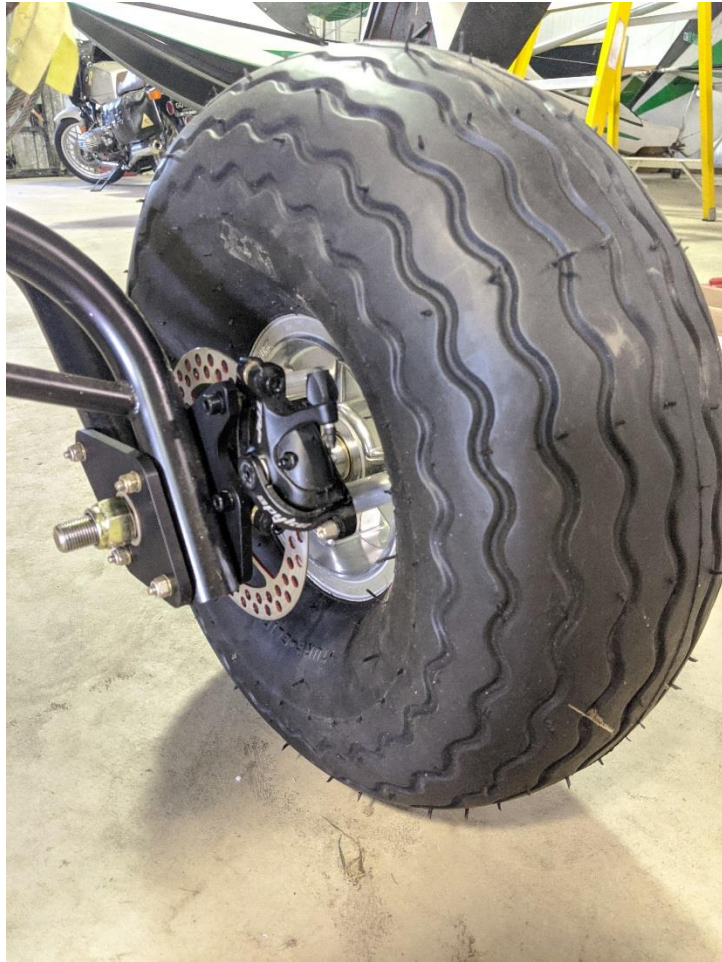
Figure 31C – Assembled Aluminum Rim, Brakes and Axle for standard 18” diameter Tundra tire
