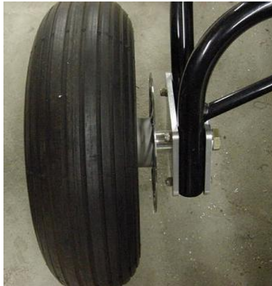
Figure 21A – Assembled Aluminum Rim and Axle for standard 12" diameter tire
