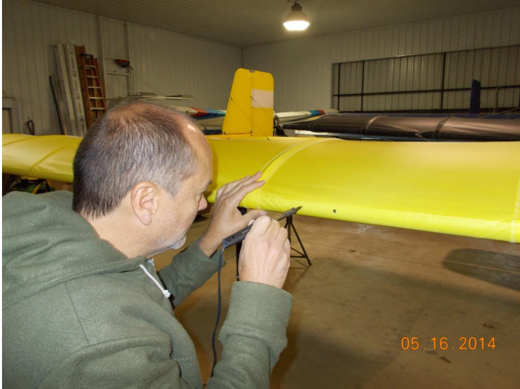
Figure 88A – Melting Holes in Fabric for Bolts
