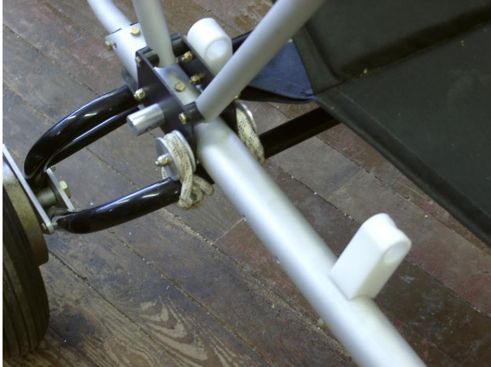
Figure 35 – Installed Delrin Support Blocks
