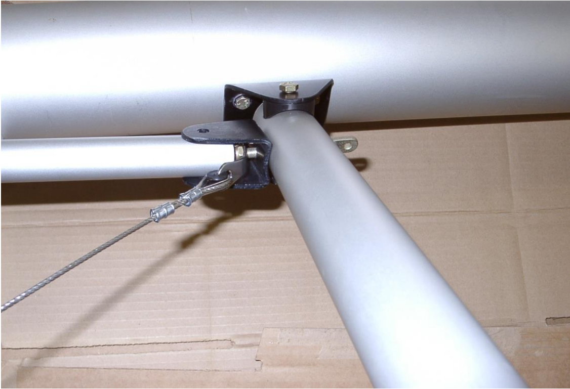
Figure 85 – Root Compression Strut (must be drilled as shown in Figure 80)
