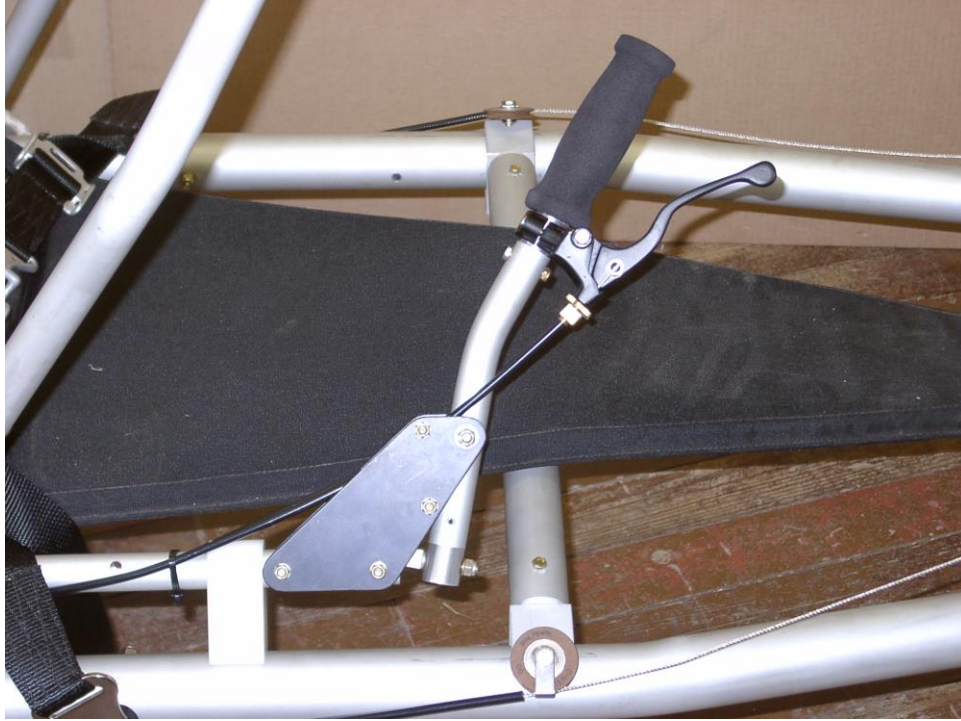
Figure 37 – Installed Control Stick (with brakes)
