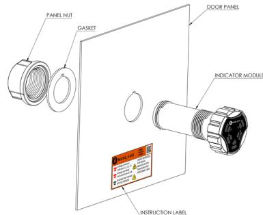
Ensure the mounting surface is clean and level. Tighten the hex nut until the VPI head rests firmly against the surface, fully compressing the Door Gasket.
