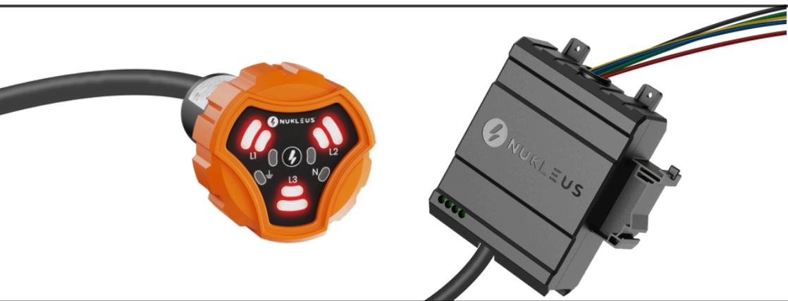
Enables qualified personnel to verify the absence of voltage with a push of a button in front of the device and provides an active indication when the absence of voltage is confirmed. The indicator module is designed to fit in a standard 30mm push buttonhole, and the Isolation Module is designed to mount on a standard DIN rail or surface mounted using screws.
