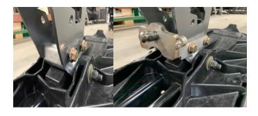
1) Remove OEM bolts (15mm) through the spindle allowing the ski to drop. (No need to relieve the pressure in the TRIO if you have one.)
