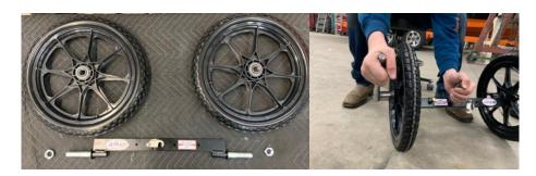
3) Using a  $1\frac{1}{16}$ " socket and a screwdriver through the pin hole for stabilization, tighten the nuts on to the axle enough for minimal wiggle room for the wheel but still allowing it to spin freely. (The wheels are identical on both sides so orientation does not matter)
