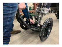
4) Pick up on the front of the ski and slide the spindle bracket into the hole in the axle. Rotate the quick clip onto the spindle bracket and the axle is locked in place. In this position you will have full handle bar rotation. Move the locking pin into the other hole and the handle bars will lock into place and the bike will be more stable.
