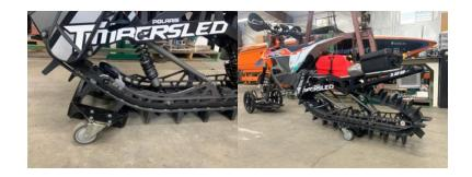
5) The Track Basket can either be installed by simply lifting the bike into the basket (we recommend having the wheels on and the pin in the lock position before attempting this method) or set the basket in front of the track and 'brap' the throttle until it is in place.
