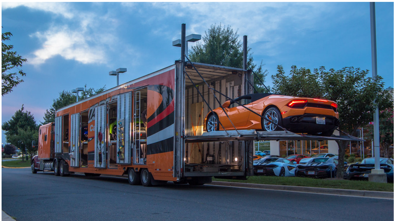
2024 KENTUCKY 53' SPLIT AXLE CUSTOM ENCLOSED CAR TRANSPORTER WITH 4 DOUBLE DOORS ON ROADSIDE AND CURBSIDE - 20,400 lbs. Tare Weight
