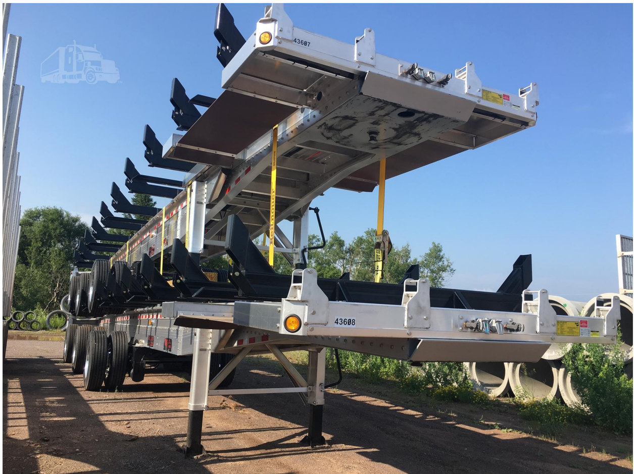
2024 REITNOUER 47' ALL ALUMINUM BUNK 12' SPREAD TRIDEM AXLE LOG TRAILER
