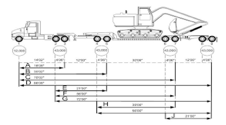
The picture above is a 2+2+2 setup and it is 95' long with tractor and and trailers. The trailer is a 65-Ton Lowboy.
