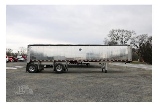
2024 MAC SMOOTHSIDE FRAMELESS 40' x 102" x 68" END DUMP w/LIFT AXLE, 24" COAL DOOR, 66-CUBIC YARDS, 12' SPREAD AXLE, 16" KINGPIN SETTING
