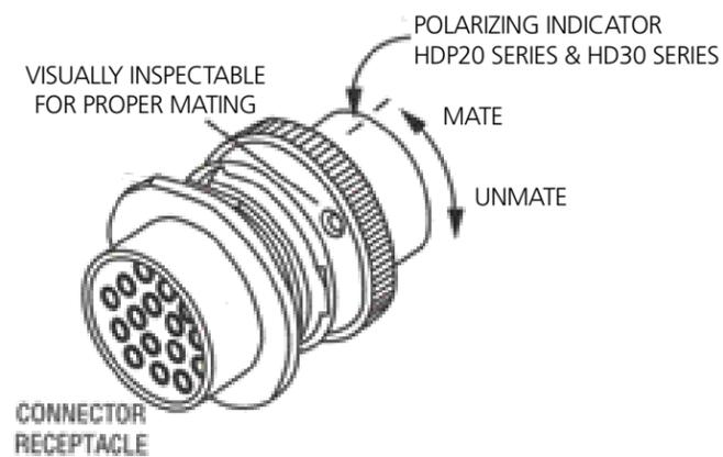
CAUTION: When mating or unmating plug and receptacle, disassemble by hand. DO NOT use pliers or any other tool.
