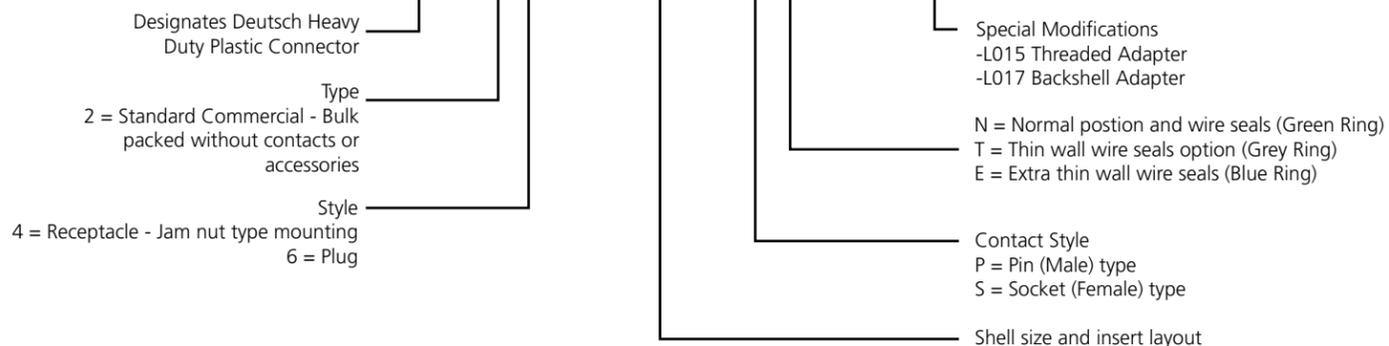
Deutsch HD30 Series contacts, sealing plugs and tooling are specified for use in the HDP20 Series. Consult factory for additional options and special modifications available.
