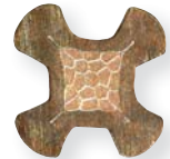
Indenter Crimp Cross-Section Across Axis
