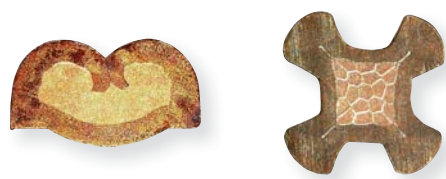
Cross section of stamped & formed and solid gas tight contact crimps
