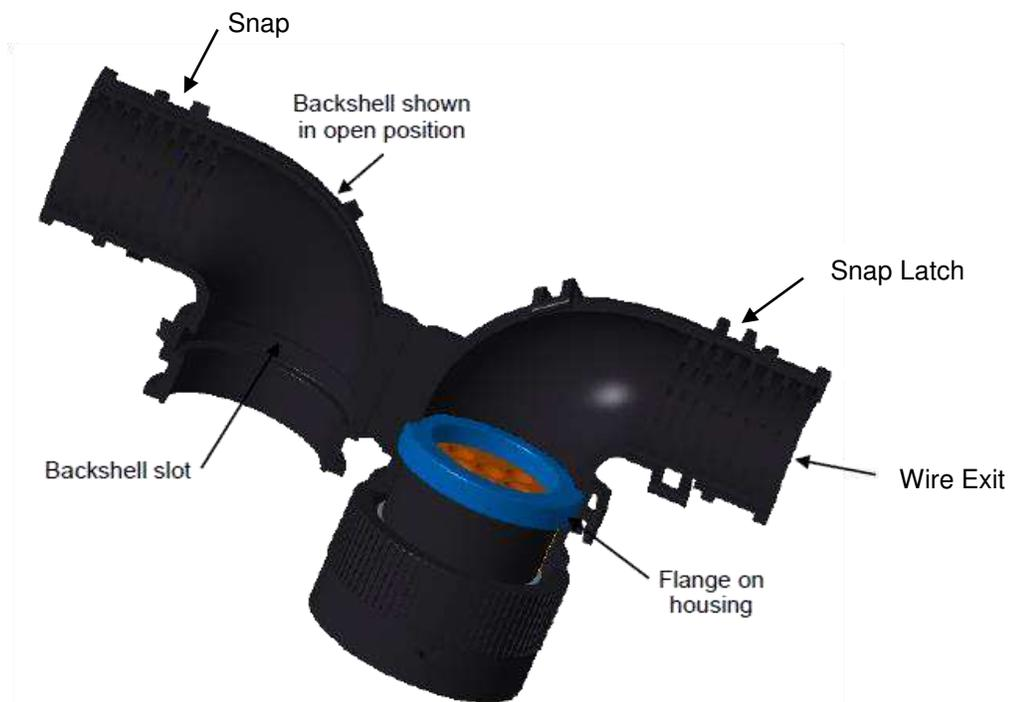
2. To close the backshell, rotate other half and line up the slots in the backshell line up with flange on housing (as described in previous step). Before snapping shut, make sure convoluted tubing (if used) is captured within the inner grooves. If no convoluted tubing is used, make sure any wires are not pinched in the backshell. There are four snaps that need to engage in order to properly snap shut the backshell.
