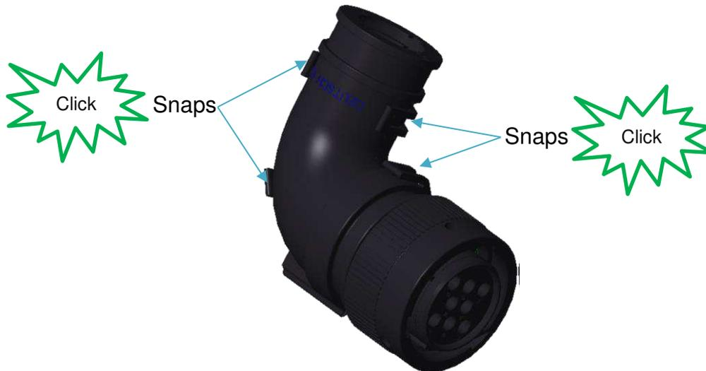
4. To remove the backshell, disengage all four snaps by wedging a DT-RT1 tool or small flat head screwdriver under the snap latch, lift until disengaged the pry the backshell open.
