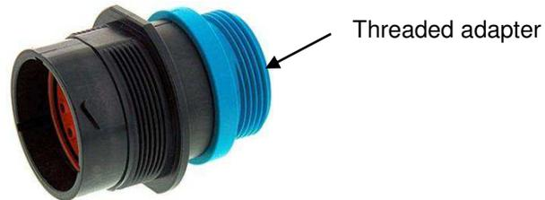
2. The second step is to screw the backshell on the back of the connector and hand tight. The connector has a threaded adapter which the backshell is threaded on.
