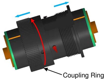
To separate the connectors uncouple the Coupling Ring counterclockwise to unmate, follow the connector as indicated by the arrows.
