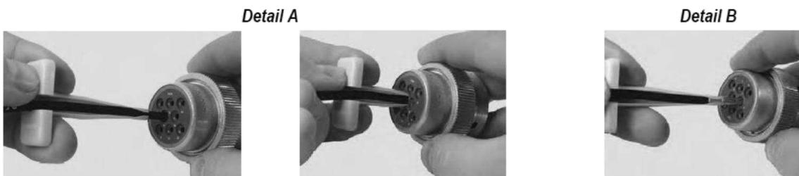
**CAUTION** Do not twist or insert the extraction tool at an angle; otherwise, damage to the cavity retention finger(s) will result.
