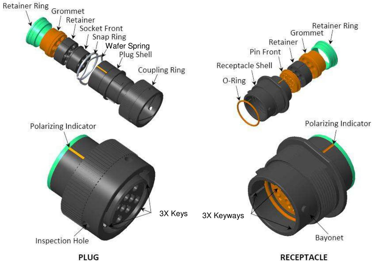
Figure 1 (Standard Configuration)
