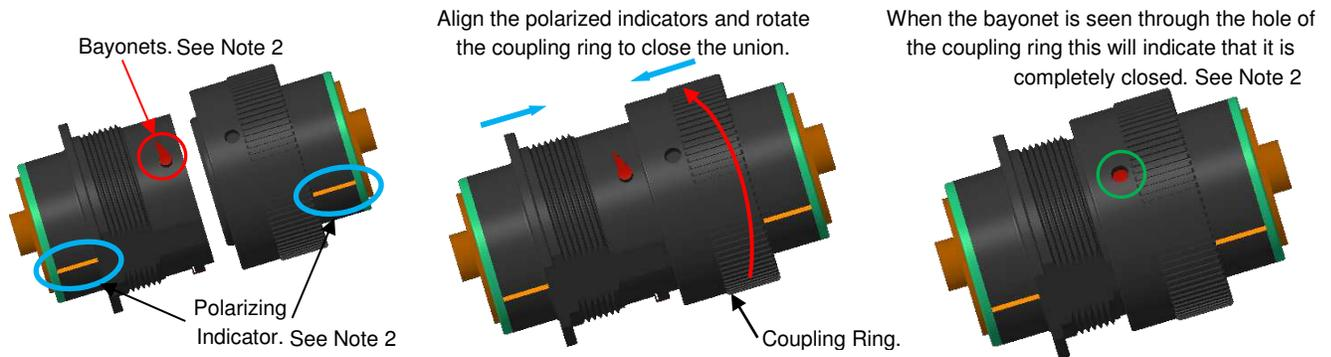
Polarized indicators serve as guides to make the connection between the connectors, each connector has an internal guide that makes the holes of the cavities are aligned but these are not visible to the naked eye, so the polarized indicators help us connect the connectors in better shape.
