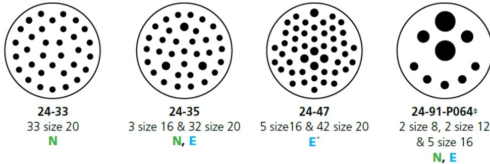
‡Without P064 modification, plug cavities 4 and 5 are internally connected.
