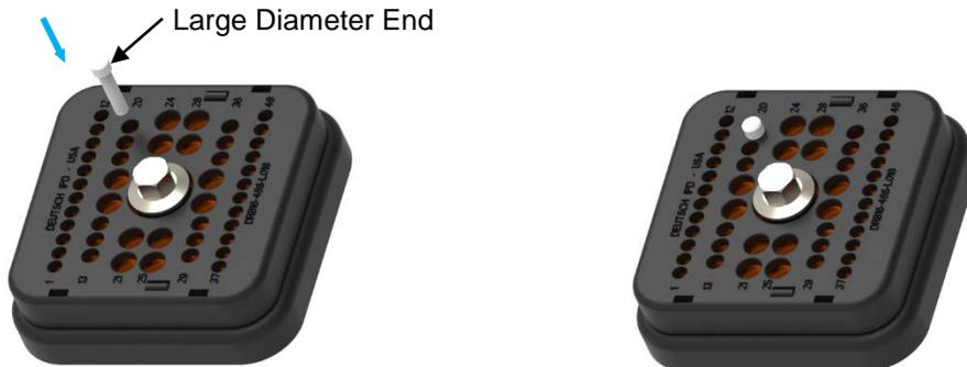
3. Visually inspect the sealing plug large diameter bottom end is flush with cap cavity opening. Do not push all the way through. Allowable distance from top of sealing plug to connector surface is shown below.
