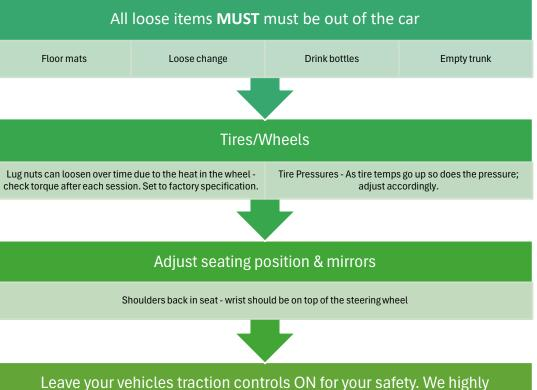
Leave your vehicles traction controls ON for your safety. We highly recommend that only expert drivers ever consider using a vehicle without traction control features.
